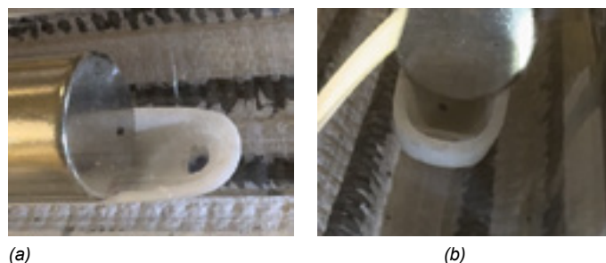
Figure 12. Quantum locking of CES-2023 at 100° C (a) and no quantum locking at 108° C (b).
