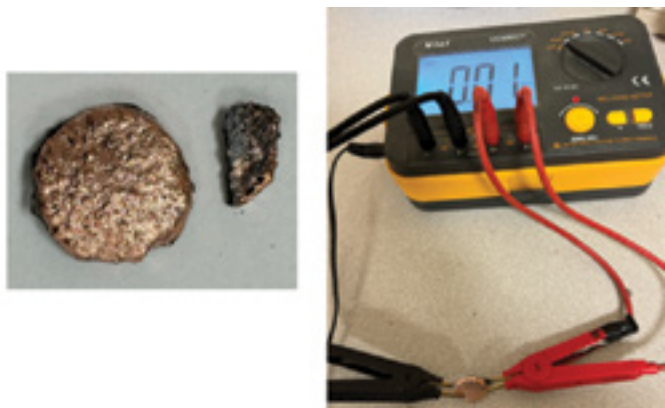
Figure 7. Copper rich sample made by 15mm pellet die. It doesn't show the Meissner effect, whereas it has very low resistance, 0.00001 \Omega , comparable to that of copper.
