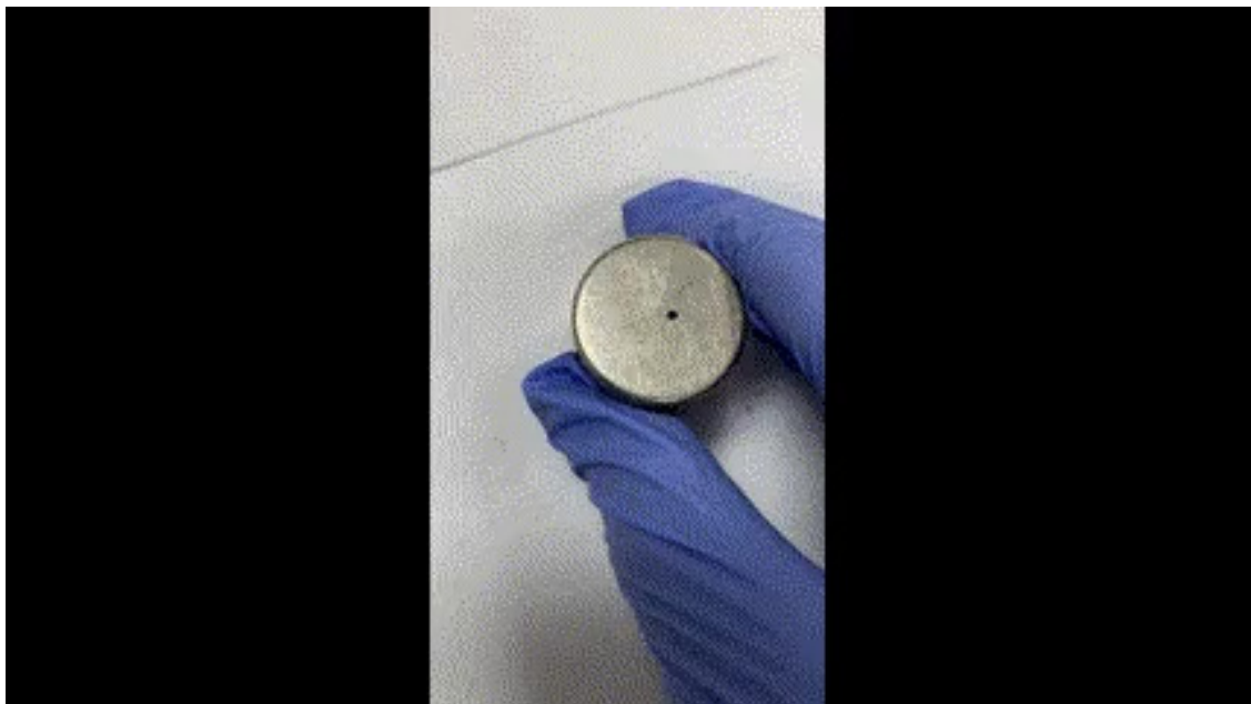
Gif file for quantum locking of CES-2023, as a magnet is rotated 180 degrees
