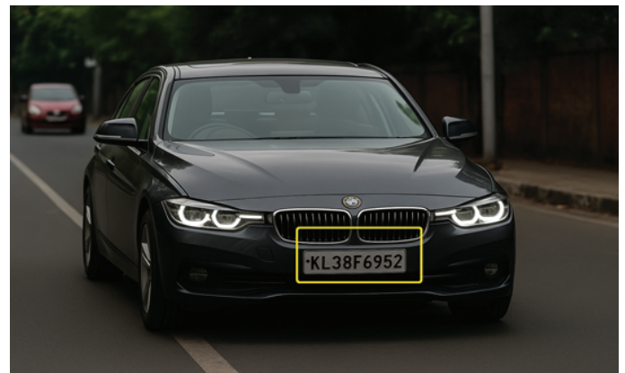
Figure 5: Example of number plate detection output using YOLOv5, showing bounding box and OCR-recognized text
