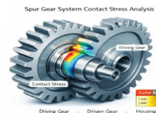
Figure 1. Contact Stress Distribution in a Spur Gear System
