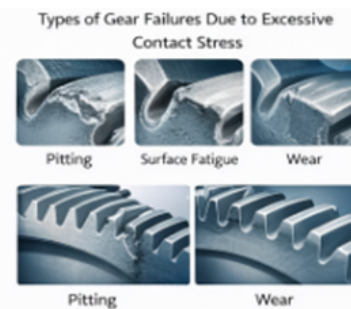
Figure 4. Types of Gear Failures Due to Contact Stress
